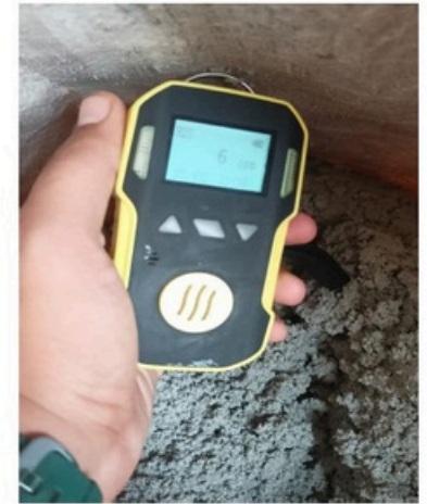
H2S meter showing H2S concentration after pressing the sludge having SYS media.
