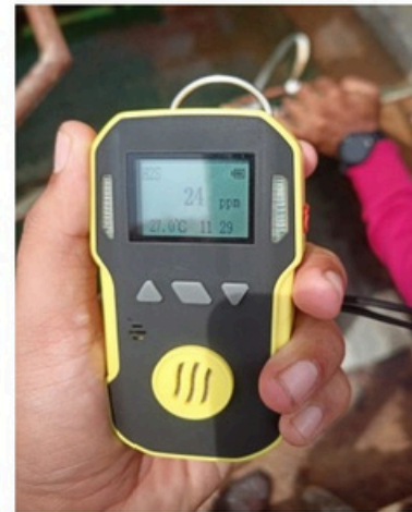
H2S meter showing H2S concentration immediately after mixing SYS media with sludge.
